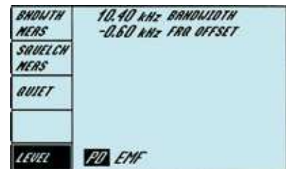
Semi-automatic search routines for squelch level, receiver bandwidth, and sensitivity perform elaborate measurements within a few seconds
